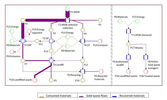
Fig. 3. Sankey diagram presenting the material flows for the LIPOR's network for 2010 modeled in Umberto®.
