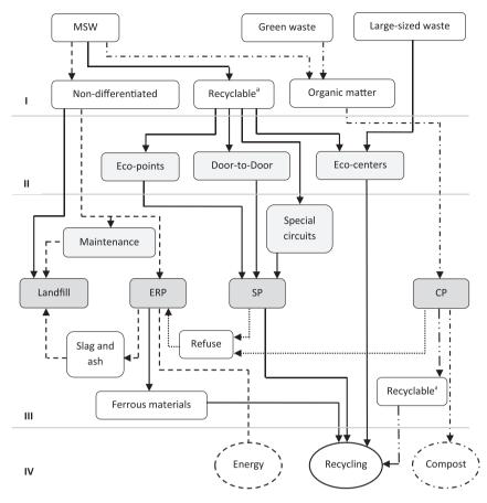
**Fig. 1.** The Integrated Waste Management System at LIPOR (adapted from LIPOR, 2009). ERP as the Energy Recovery Plant, SP as the Sorting Plant and CP as the Composting Plant. I – Citizen: production and disposal II – Councils: production and disposal III – LIPOR: valorization and treatment IV – Clients: products and resources <sup>a</sup> Recyclable are the wastes that can still be converted into valuable materials.
