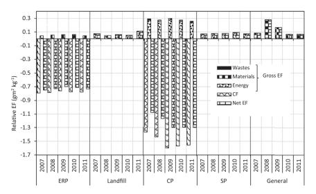
Fig. 7. Relative EF estimates for the four waste treatment processes and general activities of LIPOR, namely Energy Recovery Plant (ERP), Landfill, Composting Plant (CP), Sorting Plant (SP) and the general activities.
