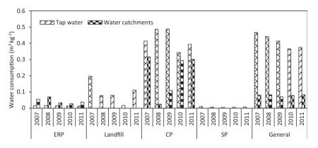
Fig. 8. Water uses at the different plants of LIPOR, namely Energy Recovery Plant (ERP), Landfill, Composting Plant (CP), Sorting Plant (SP) and the general activities.
