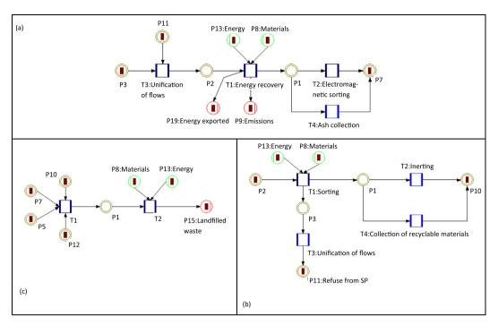
Fig. 4. Subnets from LIPOR's main network for 2010 modeled in Umberto<sup>®</sup>: (a) Energy Recovery Plant; (b) Sorting Plant; (c) Landfill.
