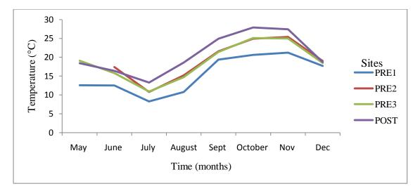
Figure 4.7: Monthly site temperature time series. PRE1: DS  $- 14.0 \pm 2.0$  °C, WS  $- 19.5 \pm 1.8$  °C; PRE2: DS  $- 18.0 \pm 2.5$  °C, WS  $- 22.2 \pm 3.2$  °C; PRE3: DS  $- 17.8 \pm 2.1$  °C, WS  $- 21.8 \pm 3.3$  °C; POST: DS  $- 19.9 \pm 2.2$  °C, WS  $- 23.1 \pm 4.4$  °C.
