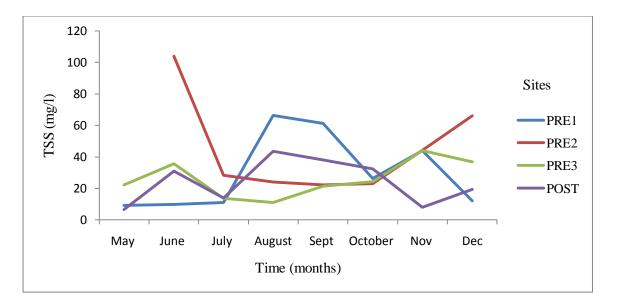
Figure 4.4: Monthly site total suspended solids time series. PRE1: DS  $-30.69 \pm 10.81$  mg/l, WS  $-27.99 \pm 15.89$  mg/l; PRE2: DS  $-40.22 \pm 15.98$  mg/l, WS  $-55.22 \pm 15.50$  mg/l; PRE3: DS  $-21.41 \pm 1.70^{**}$  mg/l, WS  $-40.49 \pm 3.55$  mg/l; POST: DS  $-27.56 \pm 5.85$  mg/l, WS  $-13.74 \pm 5.68$  mg/l. \*\*Significant at 5% significance level.
