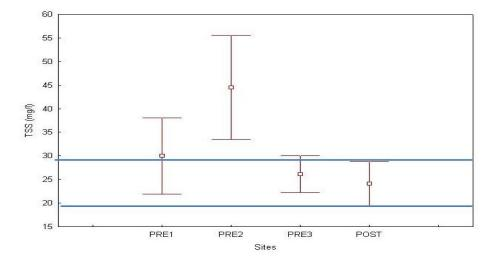
Figure 4.3: Mean site total suspended solids values for the nine months of sampling (n = 9). Model P > 0.05. The blue line represents the acceptable range of TSS of aquatic environments in the Klip River catchment of 20-30 mg/l (In-stream water quality guidelines for the Klip River catchment (IWQGKRC) 2003).
