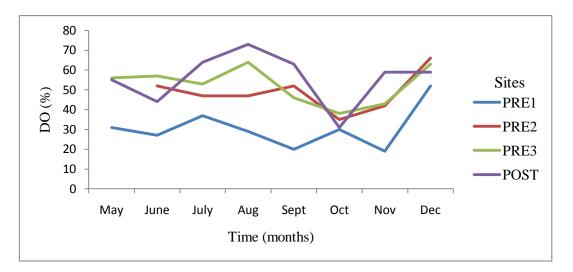
Figure 4.14: Monthly site % dissolved oxygen saturation time series. PRE1: DS  $-29.00 \pm 2.27$  %, WS  $-35.50 \pm 16.50$  %; PRE2: DS  $-46.60 \pm 3.11$  %, WS  $-54.00 \pm 12.00$  %; PRE3: DS  $-52.30 \pm 3.73$  %, WS  $-53.00 \pm 10.00$  %; POST: DS  $-55.00 \pm 6.23$  %, WS -59.00%.
