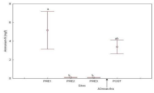
Figure 4.18: Mean site ammonium-N concentrations for nine months of sampling (n = 9). Model P < 0.01. Groups a and b are different.
