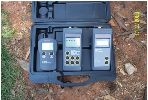
Figure A5: Meters used for measuring pH, EC and DO.
