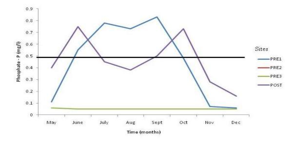
Figure 4.21: Monthly site phosphate-P time series. PRE1:  $DS - 0.58 \pm 0.11^{**}$  mgP/l,  $WS - 0.07 \pm 0.01$  mgP/l; PRE2: DS - 0.05 mgP/l, WS - 0.05 mgP/l; PRE3: DS - 0.05 mgP/l, WS - 0.05 mgP/l; POST:  $DS - 0.54 \pm 0.07$  mgP/l,  $WS - 0.22 \pm 0.06$  mgP/l. \*\*Significant at 5 % significant level. The black line represents the upper limit for the acceptable range for phosphate in the Jukskei River catchment (City of Johannesburg, 2009).
