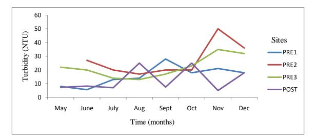
Figure 4.2: Monthly site turbidity time series. PRE1: dry season mean (DS)  $- 14.43 \pm 3.26$  NTU, wet season mean (WS)  $- 19.50 \pm 1.50$  NTU; PRE2: DS  $- 20.80 \pm 1.66^{**}$  NTU, WS  $- 43.00 \pm 7.00$  NTU; PRE3: DS  $- 18.17 \pm 1.70^{**}$  NTU, WS  $- 33.50 \pm 1.50$  NTU; POST: DS  $- 13.33 \pm 3.69$  NTU, WS  $- 11.50 \pm 6.50$  NTU. \*\*Significant at 5% significance level.
