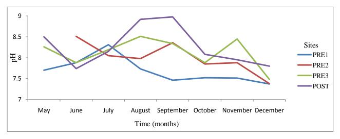
Figure 4.9: Monthly site pH time series. PRE1: DS  $-7.77 \pm 0.12^*$ , WS  $-7.45 \pm 0.05$ ; PRE2: DS  $-8.18 \pm 0.12^*$ , WS  $-7.65 \pm 0.25$ ; PRE3: DS  $-8.18 \pm 0.10$ , WS  $-8.00 \pm 0.50$ ; POST: DS  $-8.40 \pm 0.17$ , WS  $-7.90 \pm 0.10$ . \*Significant at 10% significance level.
