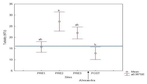
Figure 4.1: Mean site turbidity values for the nine months of sampling (n = 9). Model P < 0.05. ±SE (standard error). Groups a and b are significantly different at P < 0.05; ab and a, and ab and b are not significantly different. The blue line represents the upper limit for the ideal turbidity of 7-16 NTU for aquatic ecosystems in the Jukskei catchment (Van Veelen 2002).
