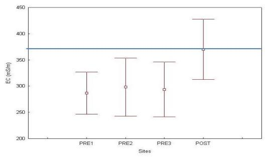
Figure 4.11: Mean site electrical conductivity for nine months of sampling (n = 9). Model P > 0.05. Blue line indicates the maximum tolerable limit for electrical conductivity in water for domestic use (DWAF 1996b).
