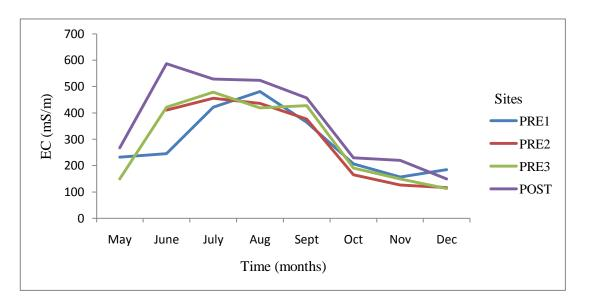
Figure 4.10: Monthly site electrical conductivity time series. PRE1:  $DS - 325 \pm 46^{**} \text{ mS/m}$ ,  $WS - 171 \pm 14 \text{ mS/m}$ ; PRE2:  $DS - 369 \pm 53^{*} \text{ mS/m}$ ,  $WS - 121 \pm 5 \text{ mS/m}$ ; PRE3:  $DS - 348 \pm 57^{*} \text{ mS/m}$ ,  $WS - 131 \pm 19 \text{ mS/m}$ ; POST:  $DS - 432 \pm 61^{**} \text{ mS/m}$ ,  $WS - 185 \pm 35 \text{ mS/m}$ . \*\*Significant at 5 % significance level. \*Significant at 10 % significance level.
