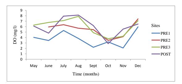
Figure 4.15: Monthly site dissolved oxygen concentration (mg/l) time series. PRE1: DS  $- 3.38 \pm 0.35$  mg/l, WS  $- 3.79 \pm 1.82$  mg/l; PRE2: DS  $- 5.11 \pm 0.47$  mg/l, WS  $- 5.48 \pm 1.52$  mg/l; PRE3: DS  $- 5.80 \pm 0.60$  mg/l, WS  $- 5.36 \pm 1.32$  mg/l; POST: DS  $- 5.69 \pm 0.79$  mg/l, WS  $- 5.72 \pm 0.37$  mg/l.
