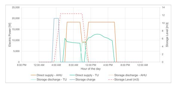
*Figure 5.17: Optimal scheduling – TES – AHU and TU operation; storage level; charge electric power.*
