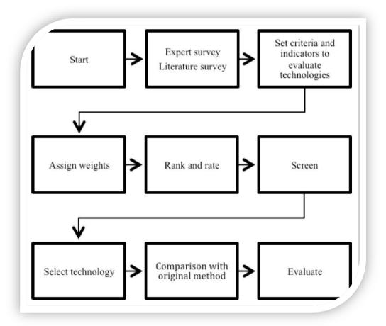
Figure 47: Process for selection of the best sewage and faecal sludge treatment technology
