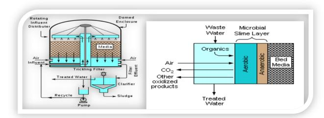
Figure 6: Trickling Filter Configuration
