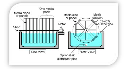
Figure 5: Schematic diagram of a typical rotating biological contactor (RBC)
