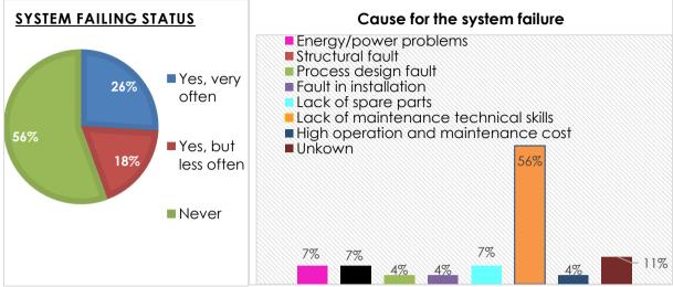
Figure 25: Causes for failing of the Sewage systems
