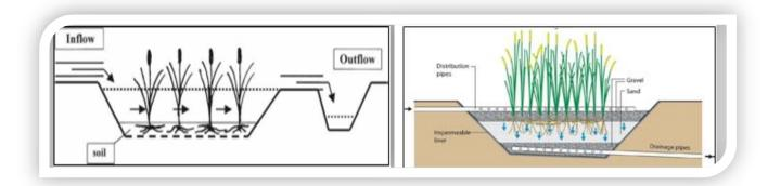
Figure 9: Constructed wetlands (surface flow at left side and subsurface flow at right side)
