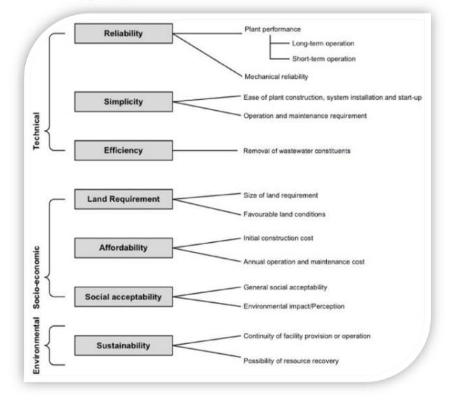
Figure 48: Factors determining the selection of appropriate wastewater treatment technologies
