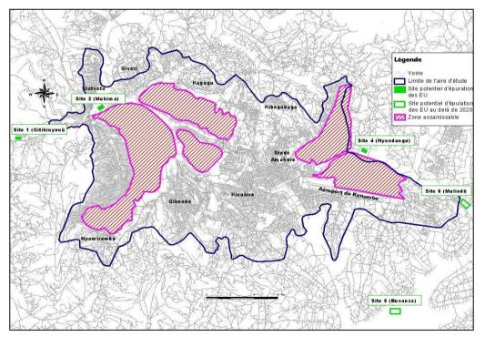
Figure 1: Area possible for the central sewage system (shaded in pink), the remaining of the zone being suitable for individual systems.
