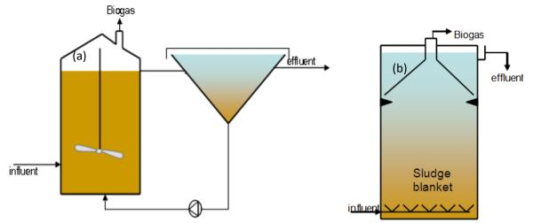
Figure 11: Anaerobic wastewater treatment using the contact reactor (a) and upflow reactor (b)
