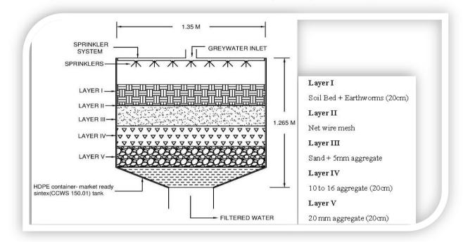
Figure 10: Vermifilter configuration
