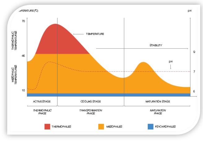
Figure 17: Stages of Biotransformation of biosolids in the composting process
