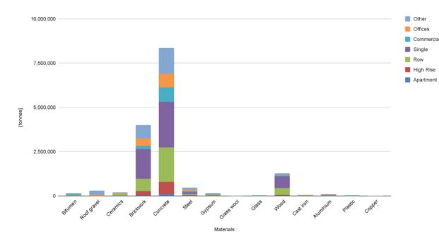
Figure 15 - Building stock by materials and building typologies
