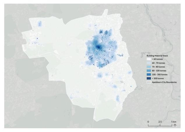
Figure 10 - Map of Building Material Stock in Apeldoorn expressed in tonnes and with an overlaid heatmap to facilitate its compression. (*interactive map* – explore it!)
