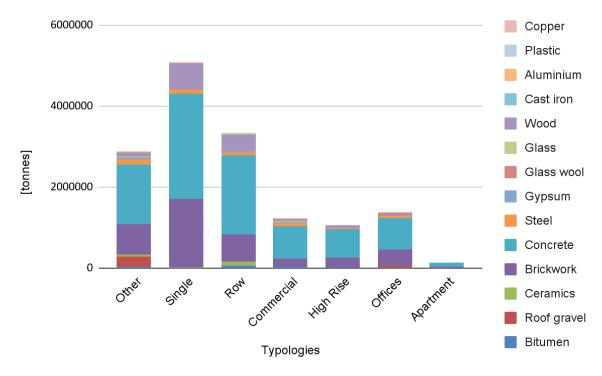
Figure 14 - Building stock by building typologies and materials
